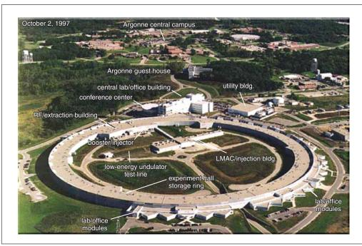
**Figure 7.13.20** X-ray Synchrotron. Aerial view of the Advanced Photon Source (APS) at Argonne National Laboratory, a so-called 3rd generation X-ray synchrotron.
