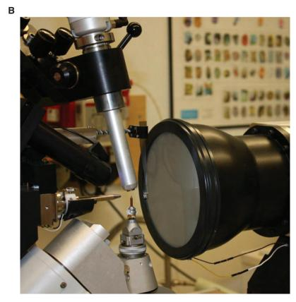
**Figure 7.13.19** X-ray generators and detectors. Two 4-circle, kappa-geometry X-ray diffraction setups currently used by researchers at Vanderbilt University. (**A**) The sealed tube Oxford Xcalibur PX2 Ultra (Oxford Diffraction), and (**B**) the rotating anode Bruker Microstar (Bruker AXS). Tube housing (Xcalibur), beam collimator, beam stop, CCD detector, crystal cooler, goniostat, goniometer head, and telescope are clearly visible.
