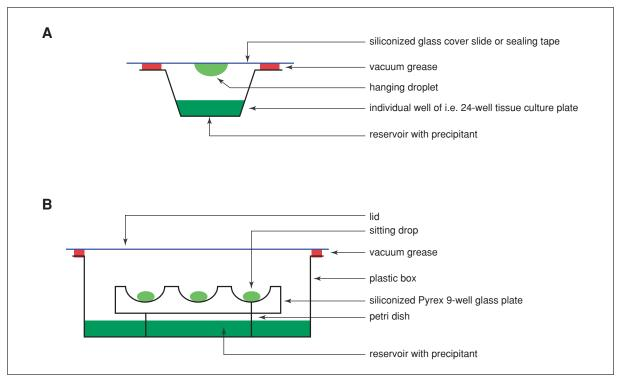
**Figure 7.13.16** Two related methods for growing single crystals of biomacromolecules. Schematic depictions of the (**A**) hanging and (**B**) sitting drop vapor diffusion techniques. The volume of the droplets is in the nL (nanodrop setting robots) to  $\mu$ L range.
