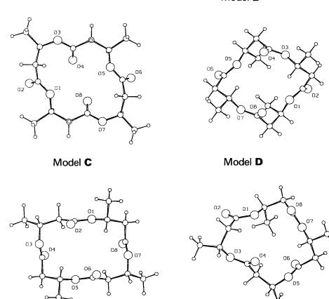
Fig. 7. Conformations of four tetrolide models after optimization by force-field methods. Models A and B were initially visually built on a graphics computer using standard bond lengths and angles and planar ester groups, model C corresponds to the crystal structure of 3-hydroxypropanoic acid [10] with four Me groups added geometrically, and model D is the best of the computer-generated models with random torsion angles.
