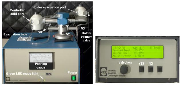
The chamber should always be left under vacuum! Cryoholders should be stored in the station under vacuum when not in use.
