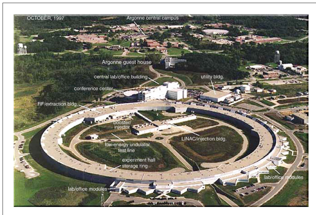
Figure 7.13.22 X-ray Synchrotron. Aerial view of the Advanced Photon Source (APS) at Argonne National Laboratory, a so-called 3rd generation X-ray synchrotron.
